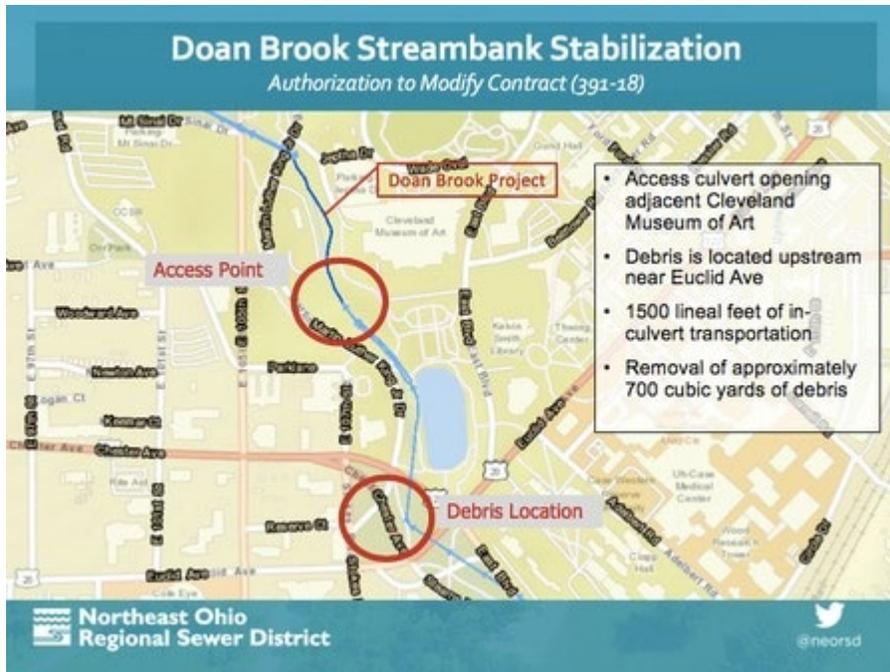
A Northeast Ohio Regional Sewer District map shows the location of debris clogging the Doan Brook culvert under a spot near Euclid Avenue (bottom circle). The clean-out will occur from the north end of the culvert at the Smith Family Gateway (top circle). Northeast Ohio Regional Sewer District
